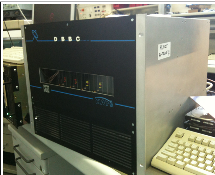
Fig.1: DBBC VLBI Backend System
