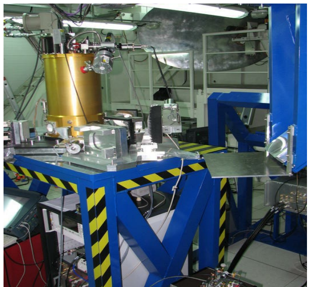
Fig.1: 3 mm receiver at the 40m cabin. The photograph shows the cryostat, mirror system (with the hot load) and the IF below the supporting structure.
