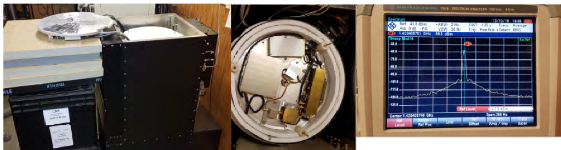
Figure 5.2: Inside of the maser and the signal (1.420405751GHz @-106dBm) from the physical part of the Maser.
