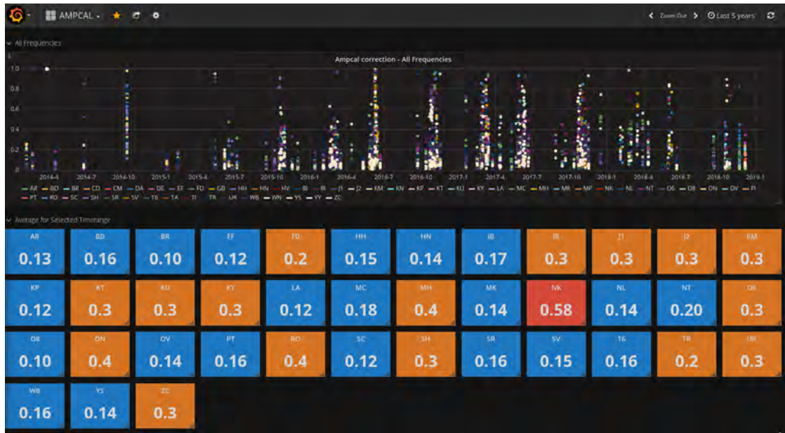
Figure 4.8: Snapshot of the web interface that allows to examine the amplitude calibration quality per station, frequency band and session.
