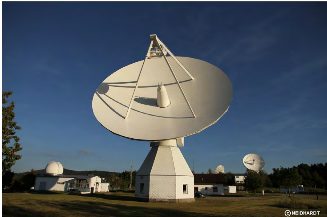
Figure 6.1: The Geodetic Observatory Wettzell with the two 13.2 m TWIN radio telescope antennas in the background on the right and the 20 m Radio Telescope Wettzell in the center.
