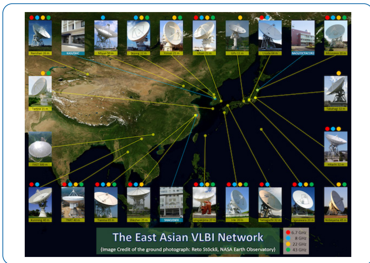
Figure 1: Concept map of the EAVN including the three correlator sites in China, Japan, and Korea. FAST 500 m telescope, which is to be used for EAVN observations at lower frequencies (< 1.6 GHz), and the Thai National Radio Telescope (TNRT), which is under construction, are also included in the map. Photograph of each radio telescope and correlator site are overlaid on 'the Blue Marble' image. Credit of the ground image: NASA's Earth Observatory.
