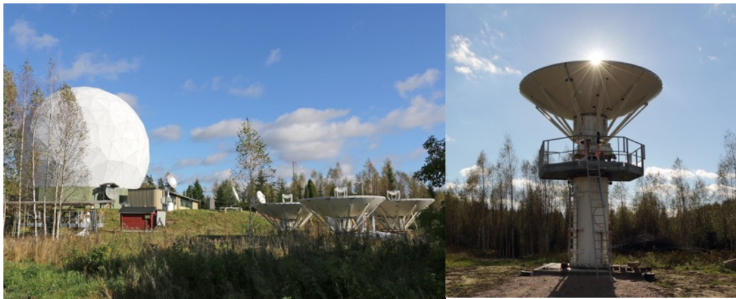
Figure 34: Left: Metsähovi in fall season. Right: The first of four Metsähovi Compact Array (MCA) antennae with a dish diameter of 5.5-metre. (Photos: Merja Tornikoski)
