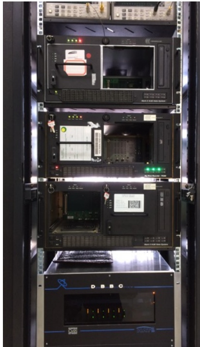
Figure 29: The new digital backend of DBBC2 in Nanshan station and the correlation fringe between Ur and T6
