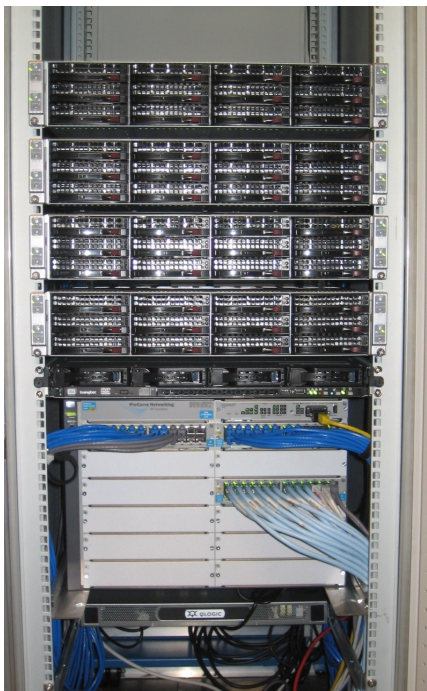
Figure 1: the SFXC cluster, consisting of four Transtec Calleo 642 servers. Each server contains four nodes, each node is equipped with two quadcore Intel Xeon 2.26 GHz E5520, giving a total of 128 cpu cores.
