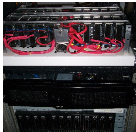
New VLBI rack with the 10 Gigabits internal switch, ibob, windows-ibob development pc, new host computer for the disk pack and the disk-pack itself.
