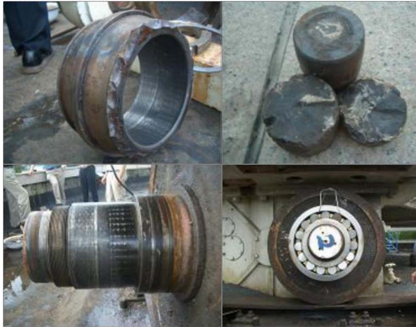
Upper panel – broken bearing; bottom panel – bearing after replacement.
