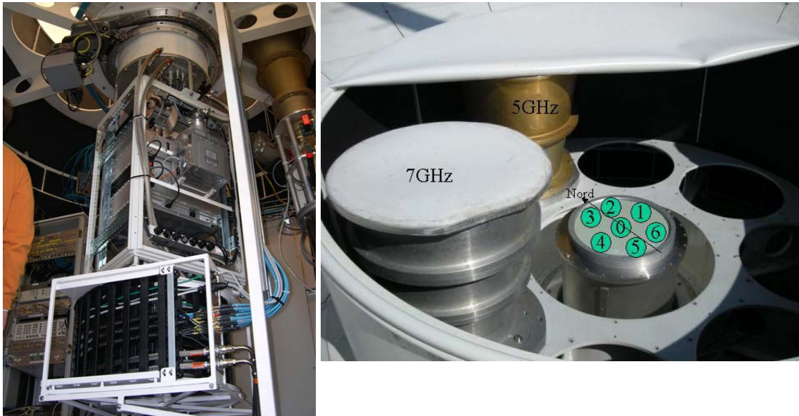
The multibeam mounted in secondary focus together with the 5 and 6 cm receivers
