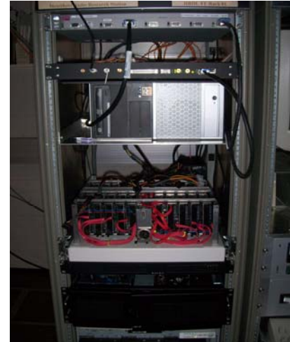
Early 2008 test of RAID controllers and port multipliers show COTS hardware for 4-6 Gbps rates to Mark5C-like 10G NAS (left). Shippable 4G-EXPREs SATA diskpack prototype on a rack-tray (right).
