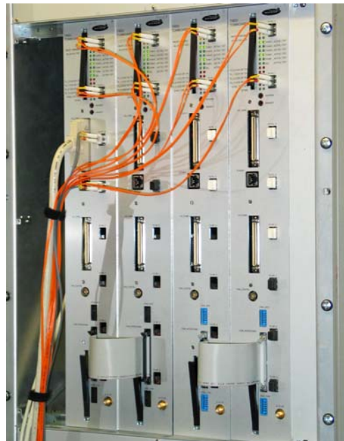
The two faces (input and output) of the new Tied Array Distribution Unit (TADU-max) that has been commissioned and taken into production during 2007-8 for use in WSRT tied array observations, including VLBI.
