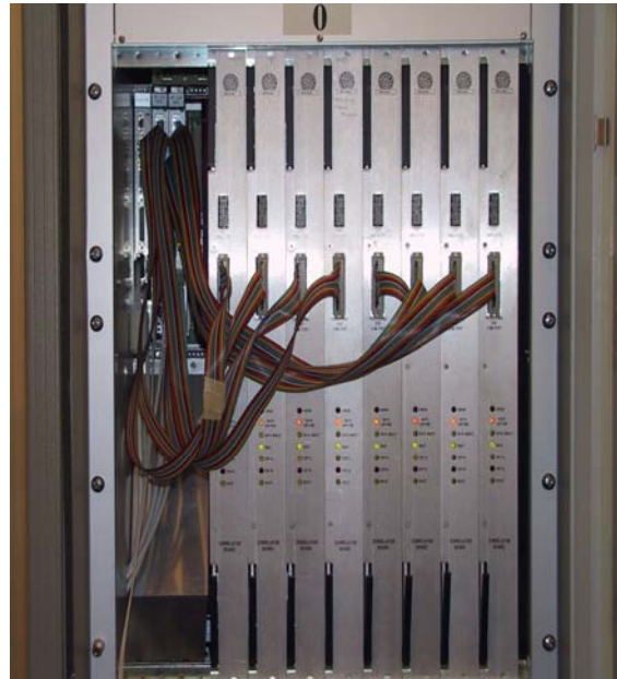
Figure 4.2: The PCInt Single Board Computers (top left) integrated with the Correlator output cards.
