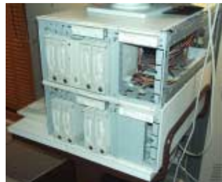
Figure 37: The two-PC prototype used to record gigabit VLBI data
