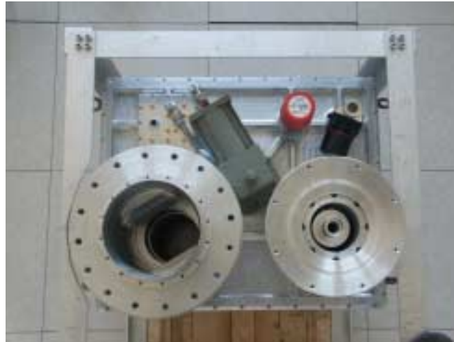
Figure 35: the new prime focus L and S/X band system for Noto.
